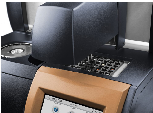
Figure 2 – Picture of the sample autosampler on the TA Instruments DSC2500. This differential scanning calorimeter (DSC) is remotely accessible for automatic and remote experiments.
